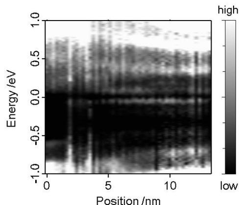
Figure1. STS spectrum of EuNW@CNT.  $dI/dV$  mapping taken along CNT axis. The left side is empty CNT area and right side is EuNW encapsulated area.
