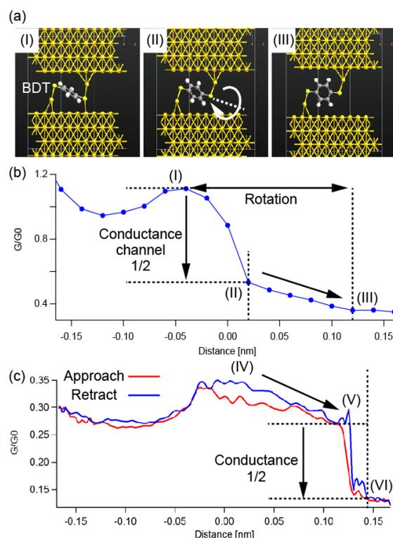
Fig. 1 Changes in the (a) molecular conformation and (b) conductance obtained by the simulation for an Au/BDT/Au junction. (c) Experimental result.
