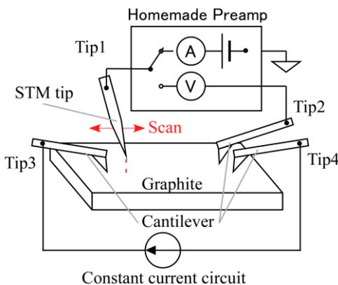
Fig. 1 Schematic of four-probe method
