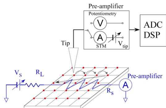
Fig. 2 Measurement concept of STM and STP
