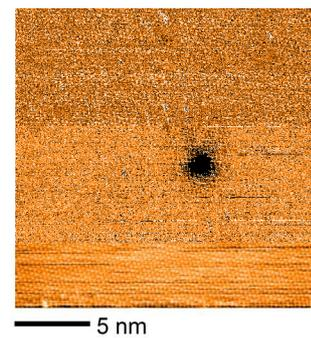
Figure 3 STM image of catalyst-assisted grown MoS<sub>2</sub> monolayer.
