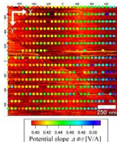
**Fig. 2:** Topographic image and mapping of potential difference between tip2 and tip3.
