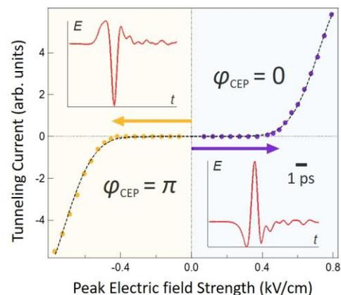
Fig. 1. Electric-field dependence of terahertz-induced tunneling current between two electrodes: a nanotip (Pt/Ir) and a sample (HOPG). Inset shows the waveforms of applied terahertz pulses.
