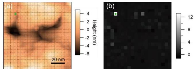
Figure 2. (a) STM topography image. (b)  $-I(V = -200 \text{ mV}) / I(V = 600 \text{ mV})$  mapping after the laser irradiation. The bright dot shows the laser-induced amorphous region.
