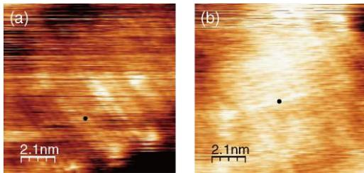
Figure 1. STM images of GST surface (a) before and (b) after laser irradiation.
