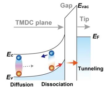
Fig. 3 Band diagram and exciton dissociation model by STM
