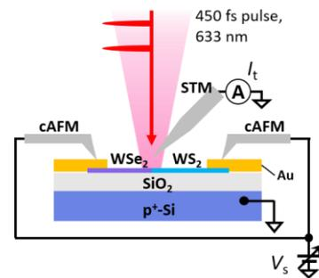
Fig. 2 Setup of time-resolved MPSTM
