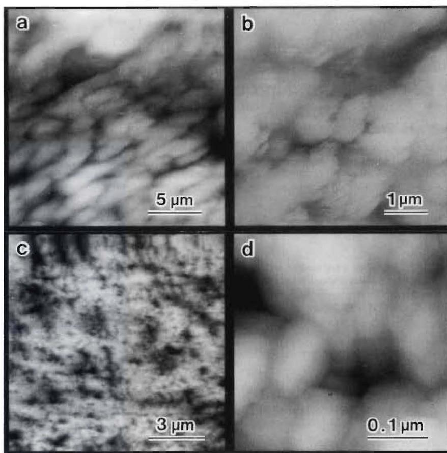
Fig. 1. Topographic images of as-grown ((a):  $20 \times 20 \mu\text{m}^2$ , (b):  $5 \times 5 \mu\text{m}^2$ ) and annealed films ((c):  $12 \times 12 \mu\text{m}^2$ , (d):  $0.4 \times 0.4 \mu\text{m}^2$ ).
