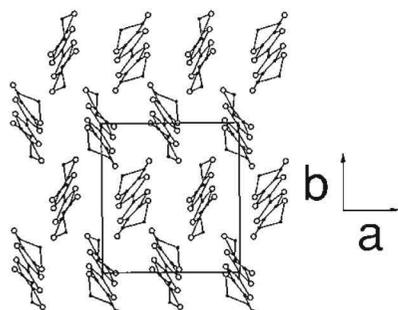
Fig. 3. Molecular arrangement of BEDT-TTF in the  $ab$ -plane of the  $\alpha$ -(BEDT-TTF) $_2$ I $_3$  crystal ( $a = 0.92 \text{ nm}$ ,  $b = 1.09 \text{ nm}$ ).
