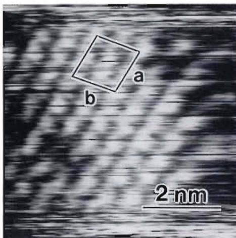
Fig. 2. Current image of the as-grown film obtained at the sample voltage of 10.1 mV ( $6.0 \times 6.0 \text{ nm}^2$ ). Unit cell is drawn for reference.
