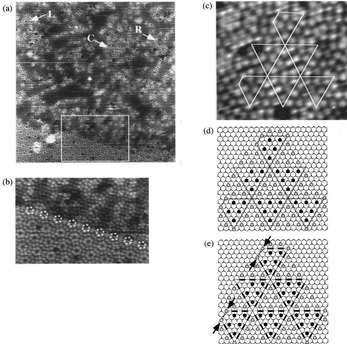
FIG. 3. (a) STM image of quenched Si(111) surface ( $V_t = -2.0$  V and  $I_t = 0.3$  nA). Corner adatoms forming corner holes of  $7 \times 7$  structure at the boundary are indicated by dots. (b) Magnification of the rectangular area in (a). (c) Magnification of the  $7 \times 7$  fragment indicated by C in (a). Two schematic models for the structure shown in (c); without [(d)] and with [(e)] stacking faults.
