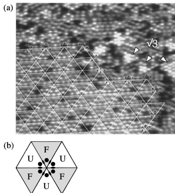
FIG. 2. (a) STM image of Si(111) surface after HBO<sub>2</sub> irradiation for 5 min at 750 °C, which includes 7×7 and disordered areas introduced by HBO<sub>2</sub> irradiation ( $V_t = -1.0$  V and  $I_t = 1.0$  nA). Corner adatoms forming corner holes of the 7×7 structure at the boundary are indicated by dots. (b) Schematic structure of a corner hole in the 7×7 structure. Ellipses represent dimers, and faulted and unfaulted half units are indicated by *F* and *U*, respectively.
