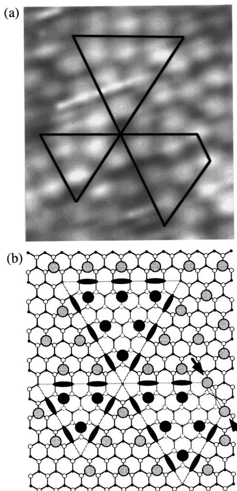
FIG. 4. (a) Magnification of the 7×7 fragment indicated by L in Fig. 3(a). (b) Schematic of the structure of (a).
