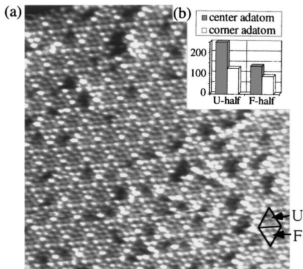
FIG. 1. STM images of Si(111) surface after HBO<sub>2</sub> irradiation for 3 min at 750 °C. Tip bias voltage  $V_t$  and tunneling current  $I_t$  are 1.0 V and 1.0 nA, respectively. The number of the reacted adatoms are shown in the inset.
