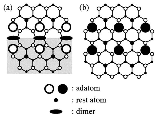
Fig. 2. Schematics of Si(111) surface structure (a) with and (b) without the stacking fault in the underlying layer. The large circles, closed circles and closed ellipses correspond to the adatoms, rest atoms, and dimers, respectively. Gray and white adatoms are considered to become dark and bright, respectively in the filled-state STM image.
