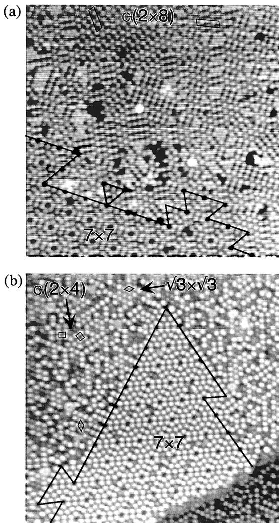
Fig. 1. STM images of the Si(111) surfaces after (a) quenching (sample bias:  $V_s = 2.0$  V, tunneling current:  $I_t = 0.3$  nA) and (b)  $\text{HBO}_2$  irradiation ( $V_s = 2.1$  V,  $I_t = 0.45$  nA).
