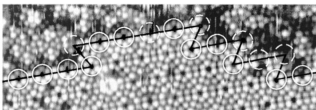
Fig. 3. Filled-state STM image ( $V_s = -2.0 \text{ V}$ ,  $I_t = 0.3 \text{ nA}$ ) of a boundary region between  $7 \times 7$  and disordered structure on a quenched Si(111) surface. The solid and dashed circles indicate the complete and incomplete corner holes, respectively.
