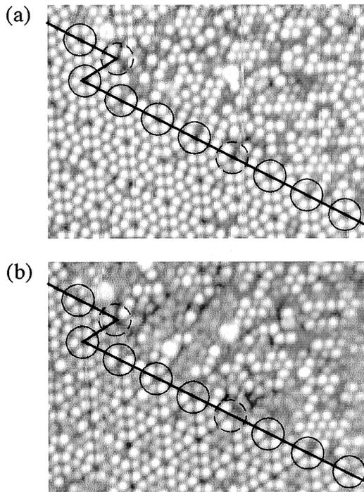
Fig. 5. (a) Empty- ( $V_s = 2.1$  V,  $I_t = 0.45$  nA) and (b) filled- ( $V_s = -2.1$  V,  $I_t = 0.45$  nA) state STM images of the boundary between  $7 \times 7$  and disordered structure on a  $\text{HBO}_2$ -irradiated Si(111) surface. The solid and dashed circles indicate the complete and incomplete corner holes, respectively.
