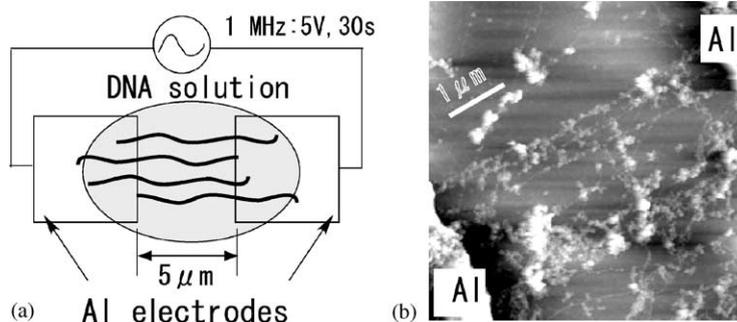
Fig. 3. DNAs bridging Al electrodes 5  $\mu\text{m}$  apart. In addition to the stretched DNA strands, there remain some unspecific structures, which may be by-products due to some electrochemical reaction.
