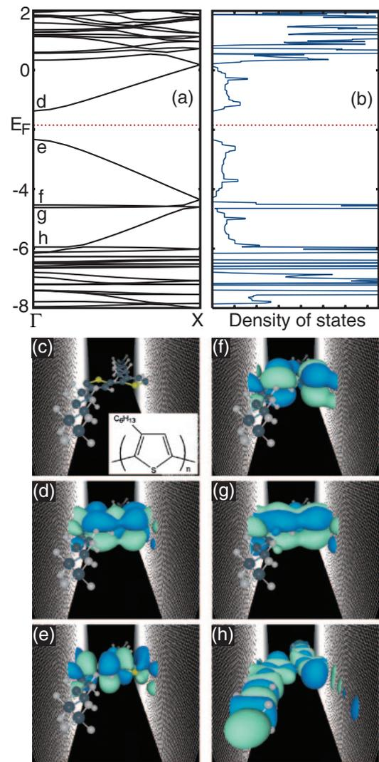
Fig. 3. Calculations of energy structures of P3HT. (a) Band structures. (b) DOS. (c) Optimized geometry. (d)–(h) Amplitudes of wave functions at  $\Gamma$ -point in (d) LUMO, (e) HOMO, (f) HOMO-1, (g) HOMO-2, and (h) HOMO-3 states. The corresponding band structures are shown in (a). The chemical structure of P3HT is shown in the inset of (c).
