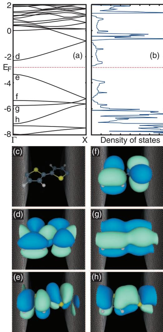
Fig. 2. Calculations of energy structures of PT. (a) Band structures. (b) DOS. (c) Optimized geometry. (d)–(h) Amplitudes of wave functions at  $\Gamma$ -point in (d) LUMO, (e) HOMO, (f) HOMO-1, (g) HOMO-2, and (h) HOMO-3 states. The corresponding band structures are shown in (a).
