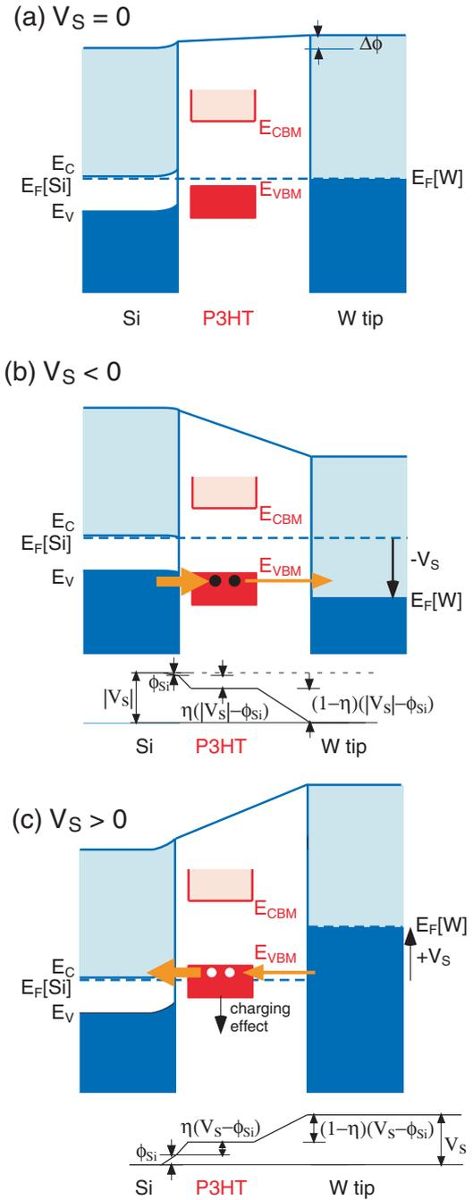
Fig. 6. Energy band diagrams in H-Si(100)/P3HT/STM tip junction.  $E_C$ ,  $E_V$ ,  $E_{CBM}$ , and  $E_{VBM}$  are energy levels of silicon-CBM, silicon-VBM, P3HT-CBM, and P3HT-VBM, and  $E_F[Si]$  and  $E_F[W]$  are Fermi energy levels of silicon and the W tip, respectively.  $\phi_{Si}$  and  $\Delta\phi$  are silicon band bending and the work-function difference between silicon and tungsten, respectively. Electrostatic potential profiles are also shown at the bottom in (b) and (c).
