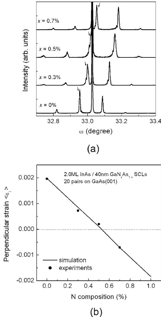
FIG. 1. (a) Symmetric (004) x-ray diffraction patterns for samples with 20 stacked layers of InAs QDs structure embedded in  $\text{GaN}_x\text{As}_{1-x}$  SCLs with  $x=0\%$ , 0.3%, 0.5%, and 0.7%. (b) Simulated (solid line) and measured (closed circle) strains in InAs/GaNAs system perpendicular to the growth axis on GaAs (001) substrate.
