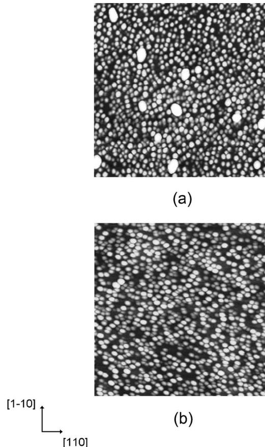
FIG. 3. AFM images of the top QD layer of 30 layer stacked InAs QDs embedded in (a) GaAs spacer layers and (b)  $\text{GaN}_{0.005}\text{As}_{0.995}$  SCLs. Scan size is  $500 \times 500 \text{ nm}^2$  in both cases.
