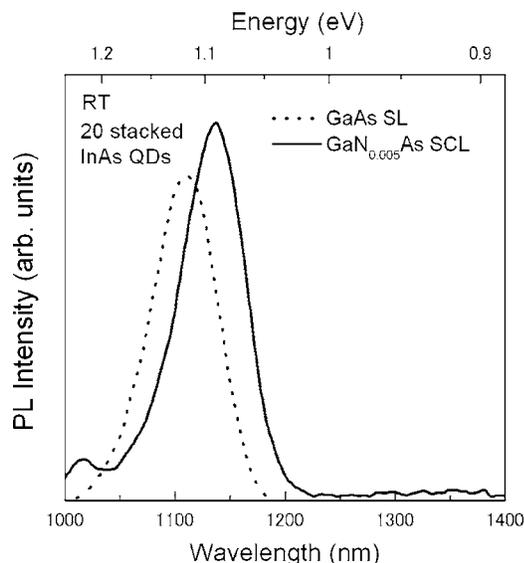
FIG. 4. PL spectra measured at room temperature from 20 stacked layers of InAs QDs embedded in GaAs spacer layers (dashed line) and GaN<sub>0.005</sub>As<sub>0.995</sub> SCLs (solid line).
