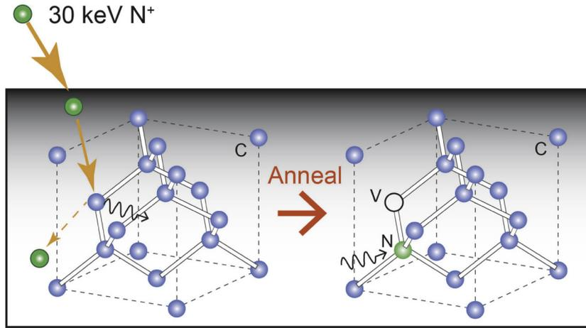
**Fig. 2.** Schematic for the production of NV centers by  $N^+$  ion implantation and subsequent annealing in diamond crystalline samples. The  $N^+$  ions implanted into diamond produce vacancies (V), which are required to make nitrogen-vacancy (NV) centers. Annealing the diamond sample induces diffusion of the vacancies, which can then be trapped by the implanted nitrogen atoms.
