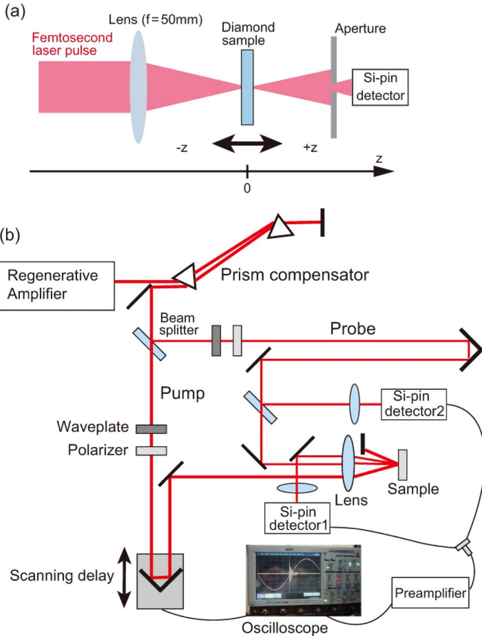
**Fig. 1.** (a) The experimental set-up for Z-scan measurement using the closed aperture mode. (b) Schematics of femtosecond pump-probe experiment with the reflection mode. The difference of the photocurrent of the two Si-pin detectors was amplified, and averaged in a digital oscilloscope using the scanning time delay at 20 Hz.
