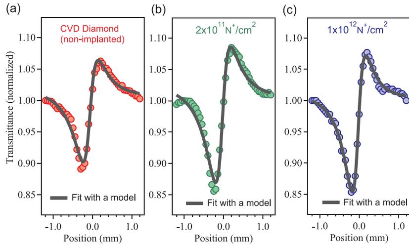
**Fig. 3.** Closed-aperture Z-scan results at  $I_0 \approx 20 \text{ mJ/cm}^2$  obtained for the pure diamond crystal and NV center introduced diamond at different dose levels, (a) non-implanted, (b)  $2.0 \times 10^{11} \text{ N}^+/\text{cm}^2$ , and (c)  $1.0 \times 10^{12} \text{ N}^+/\text{cm}^2$ . The black solid lines represent the fit to the data using Eq. (2).
