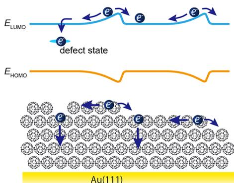
**Figure 8.** Model for the observed electron motion. Schematic illustration showing the ultrafast electron motion in the  $C_{60}$  multilayer sample influenced by the local modulation of the band structure and the in-gap state around surface steps and defects.
