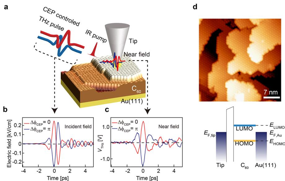
**Figure 1.** Measurement system and sample. (a) Schematic illustration of the measurement setup. (b) Waveform of incident electric field for  $\Delta\Phi_{\text{CEP}} = 0$  and  $\pi$ . (c) Waveform of near-field electric field for  $\Delta\Phi_{\text{CEP}} = 0$  and  $\pi$ . (d) STM image of the sample. (e) Band diagram of the STM tunnel junction at equilibrium ( $E_{\text{LUMO}} - E_{\text{F,Au}} = 0.9$  eV,  $E_{\text{F,Au}} - E_{\text{HOMO}} = 2.2$  eV).
