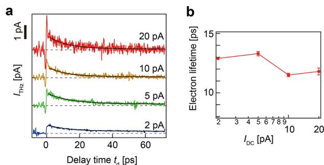
**Figure 4.** Effect of electron extraction. (a) Delay time dependence of the THz current at different set point currents  $I_{\text{DC}}$  ( $\Delta\Phi_{\text{CEP}} = 0$ ,  $V_{\text{DC}} = -3.0$  V, IR: 20 mW). (b) Set point current dependence of the lifetime shown in (a).
