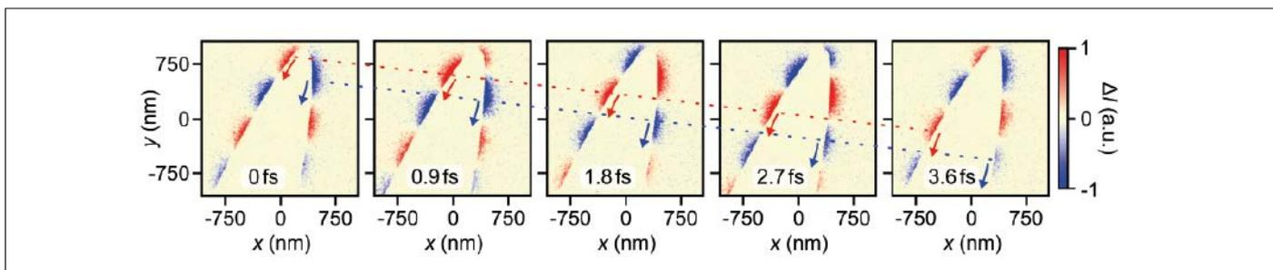
Fig. 3: Movies of light-matter interactions with the attosecond electron microscope. Plasmon-polaritons are excited with a laser on a tungsten needle and propagate downwards along the surface. Attosecond electron microscopy provides a movie of the electric fields (blue, red) in space and time.
