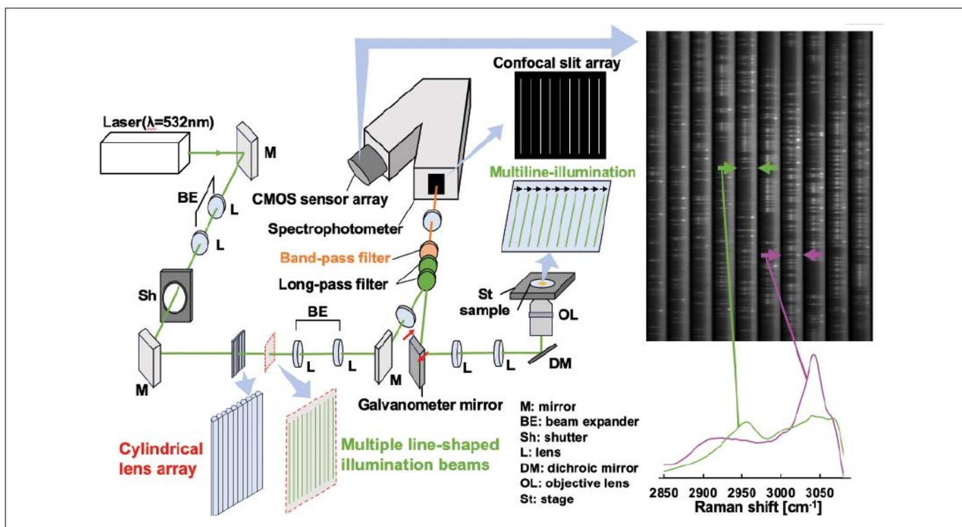
Fig. 2: A schematic diagram of the multiline-illumination Raman microscope equipped with a confocal slit array. Each Raman band in the Raman hyperspectral image corresponds to the CH region, where characteristic Raman peaks from polystyrene (magenta) and polymethylmethacrylate (green) beads are found at 2,953 and 3,047  $\text{cm}^{-1}$ , respectively.
