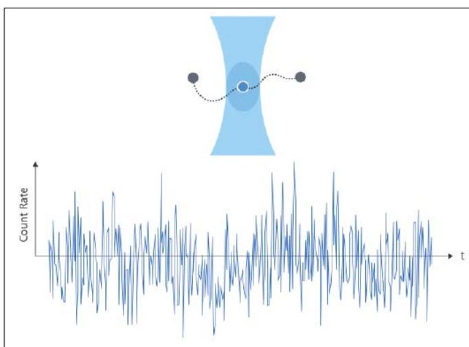
Fig. 1: A stationary excitation volume, created by an objective lens focused laser beam (top) is positioned in a sample. Fluorescence intensity fluctuations are recorded for this spot over several seconds, resulting in an intensity trace measurement (bottom).
