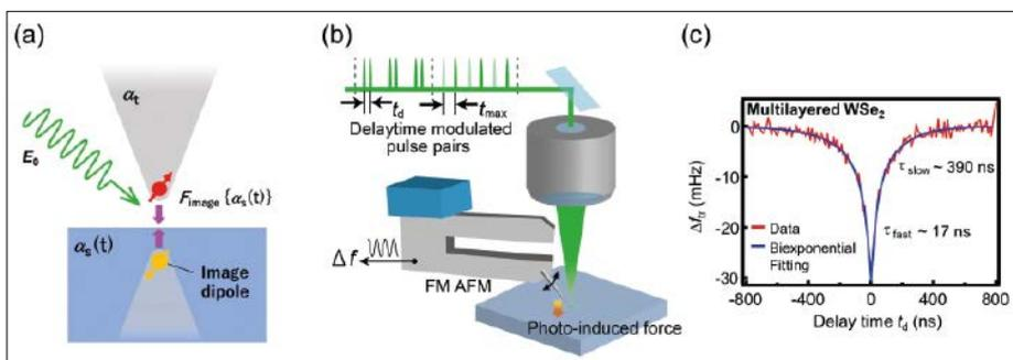
**Fig. 4:** (a) Dipole-dipole interaction mechanism.  $\alpha_t$ ,  $\alpha_s$ , and  $E_0$  are the complex effective polarizabilities of the tip and sample, the incident light electric field vector, respectively. (b) Schematic of tuning-fork-type time-resolved FM AFM setup. (c) Time-resolved signal obtained for a multilayer  $WSe_2$  sample and fitting results. [14]
