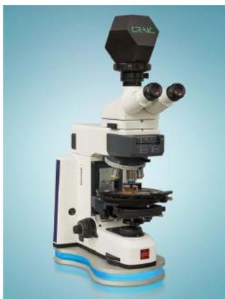
The Geolmage microscope imaging photometer by Craic Technologies is a high-performance instrument with advanced optical capabilities for analyzing materials at a
