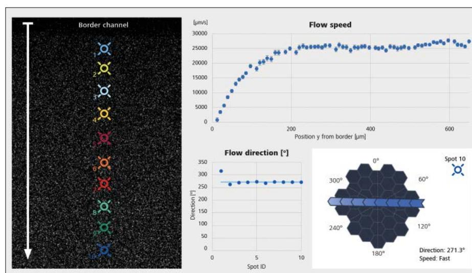
Fig. 4: Analysis of flow characteristics in a microfluidics channel. The Automated Sequential Injection System Aria by Fluigent was used to pump a rhodamine 110 solution through a microfluidic flow cell ( $1000 \mu\text{m}$  channel width).
