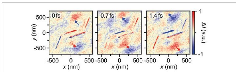
Fig. 4: Optical field-cycle dynamics in a dielectric metamaterial. The functionality of the individual nanoresonators and their collective response in the far-field is measured with our attosecond electron microscope as a movie in space and time.
